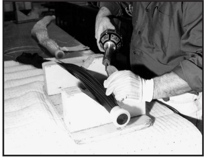
FIGURE 2 —Apply heat to the end of the tube with a plastic welding gun.
